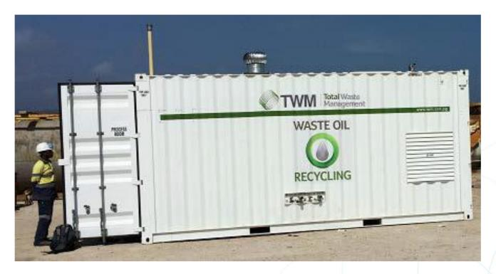
Figure 8 Containerised used oil processing and fuel blending unit (PNG)<sup>35</sup>
